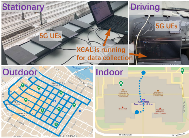
Fig. 2: The top figures depict our measurement setup. The bottom figures show the selected measurement routes and stationary experiment locations (marked by the green icons).
